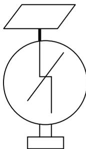
3. Charge the golf tube with the fur and touch the tube to the zinc to charge the zinc and electroscope. Electrons are transferred to the electroscope.
