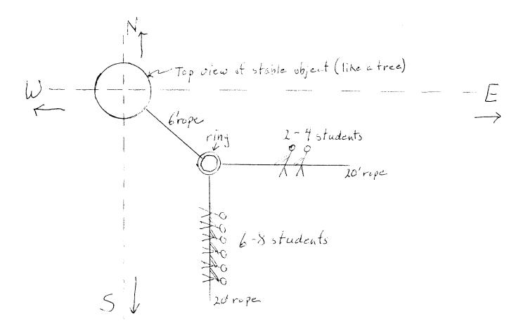
Theory: This activity will show direction and relative size of a resultant formed from simultaneously applying two forces to a metal ring.
