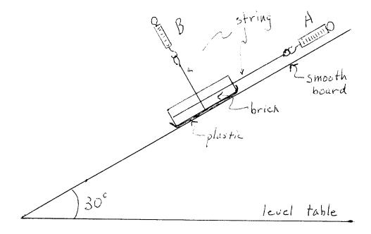
Theory: One force vector can be made up from two or more forces (or, two forces can produce the same result as one force).
